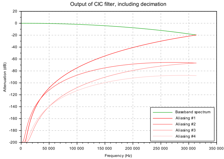
Figure 3: Decimation with a CIC filter, R = 16 , N = 5 and M = 1 - Frequency response after decimation (spectrum aliasing)
